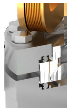
Figure A.1 | Helicoflex sealing of the 2D-MOT cell illustrated by a CAD model.
